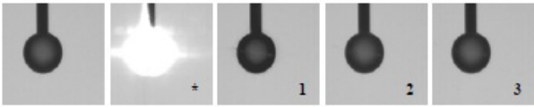
FIG. 28 Recording of the effects produced at resonant interaction on the droplet containing R6G at 10^{-3}M in distilled water by the laser beam sent horizontally and focused in the centre of it (position 1 Figure 2). E_4 = 1 mJ Movie-23 (4,9 MB).
