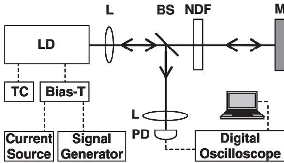
**Figure 1.** Setup of the LD driven by a periodic signal generator. PD, BS, NDF, M and TC stand for the photodiode, beam-splitter, neutral density filter, mirror and temperature controller, respectively.
